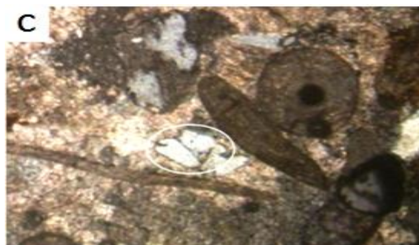
Plate 2c. Planar contact between quartz grains in MF5, 10x
