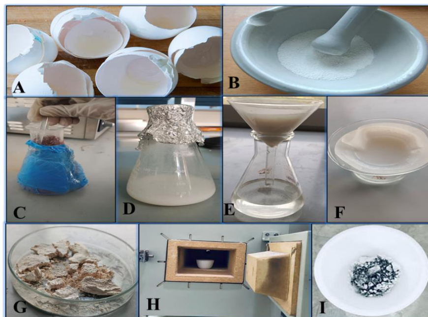
Figure 4: Synthesis of CaO nanoparticles (A) Raw hen eggshells, (B) Eggshells powder, (C) Mixture of HCl and NaOH containing eggshell powder (D) Condensation reaction after 24 hours (E) Filtration process (F) Washing of obtained product with distilled water (G) oven drying of filtered gel (H) Muffle furnace calcination of dried gel (I) Calcinated gel powder (CaO Nanoparticles)
