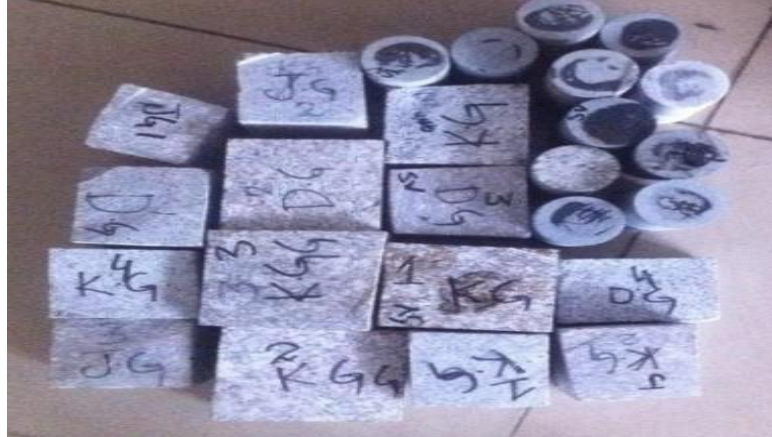
Figure 3: Figure showing prepared cubes and cylinder samples for lab testing
