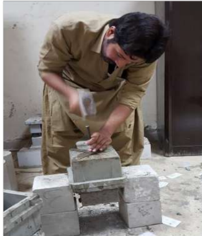
Figure. 5: Demoulding of cubes
