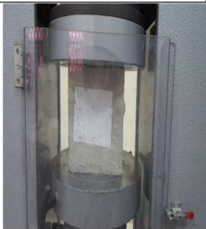
Figure. 7: Compressive test of cube
