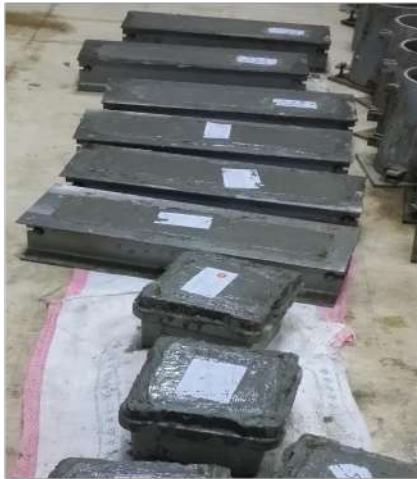
Figure. 4: Casting of concrete specimen
