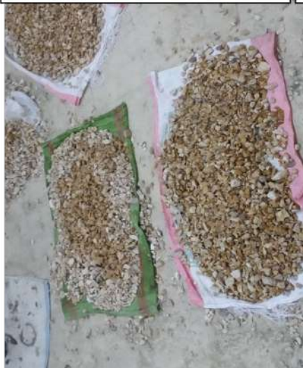
Figure. 1: Saturated surface drying of aggregates
