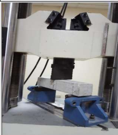
Figure. 8: Flexure test of beams
