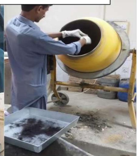
Figure. 3: Addition of Hair Fiber in concrete mix
