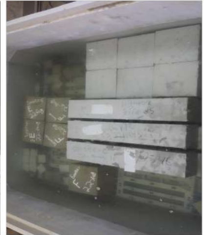
Figure. 6: Curing of concrete specimen
