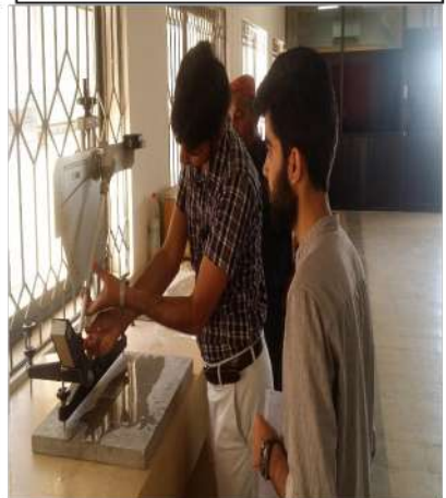
Figure. 9: Skid resistance test of slab specimen
