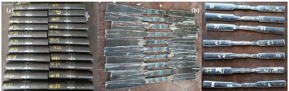
Figure 1: (a) Welded specimens, (b) Cut specimens for Tensile testing, and (c) fractured specimens after tensile testing.
