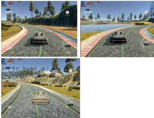
Fig. 5. Actual Results of Simulator showing middle predicted line and car following that line
